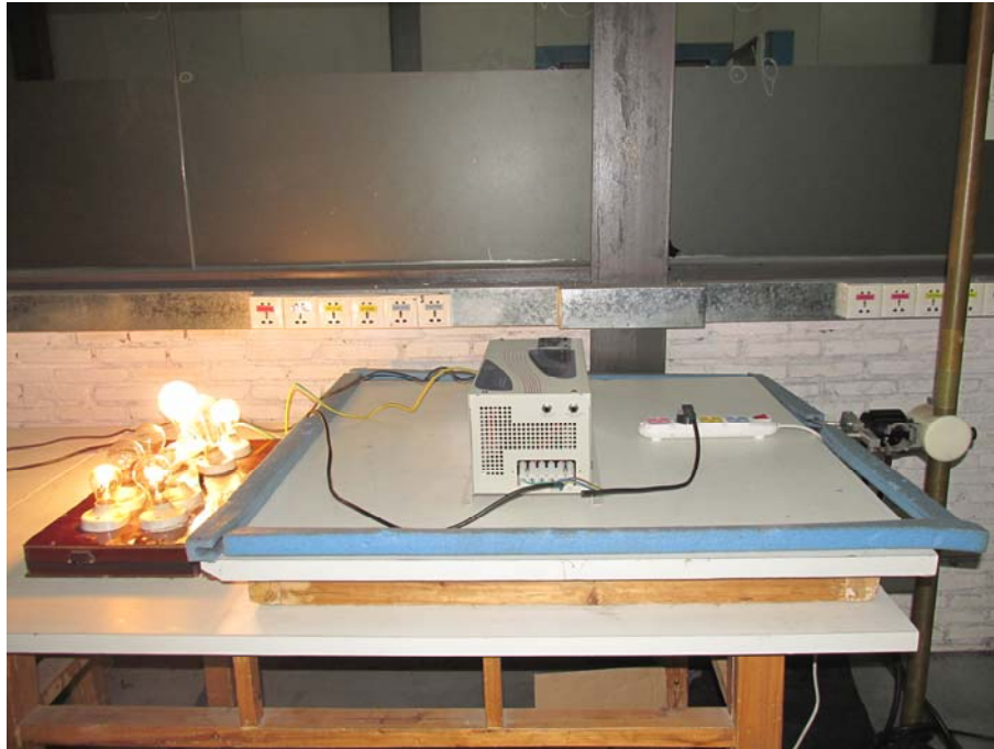
16.9. Photo of Magnetic Field Immunity Test
