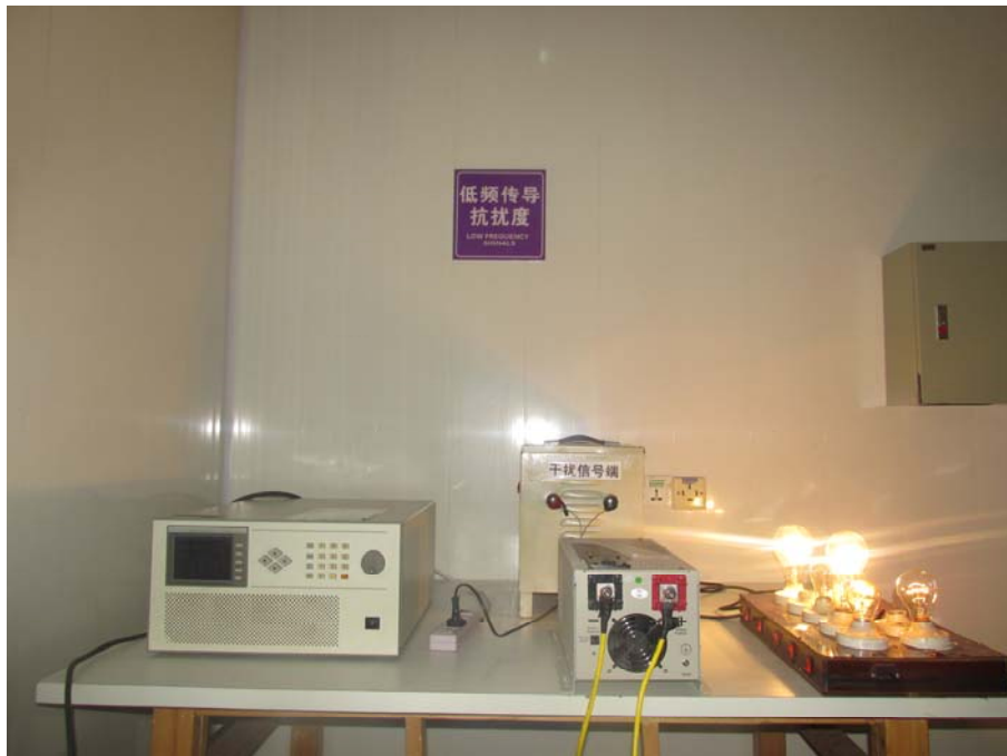
16.10. Photo of Low Frequency Signals Test
