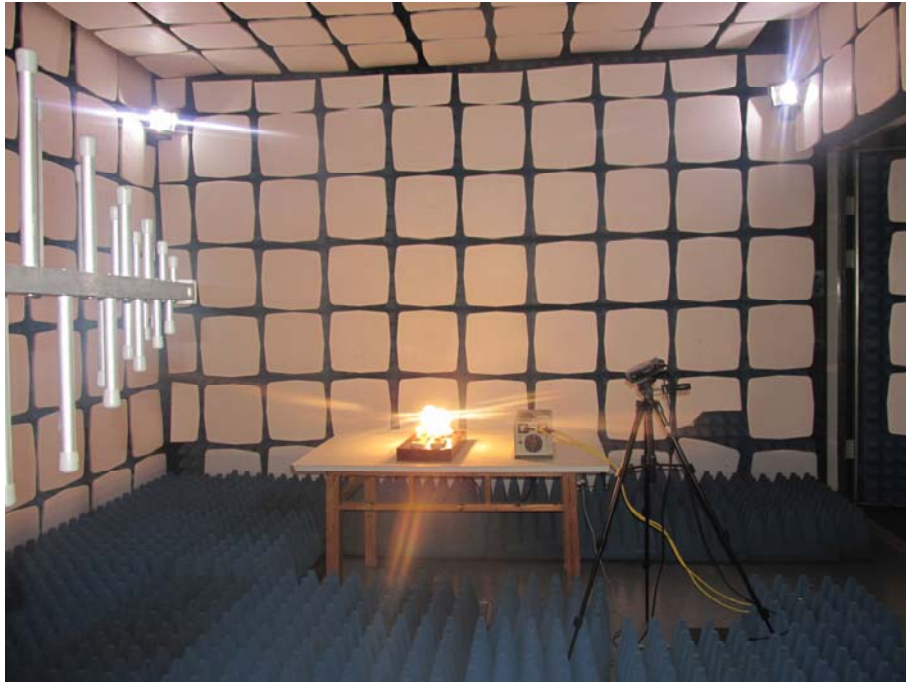
16.5. Photo of RF Field Strength susceptibility Test
