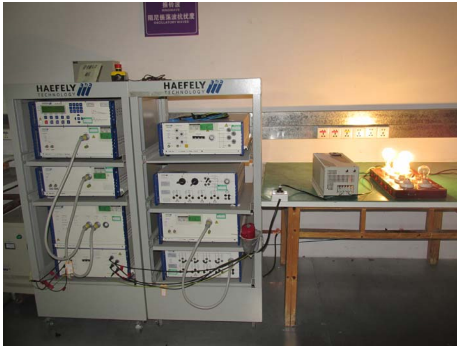
16.7.Photo of Surge Test
