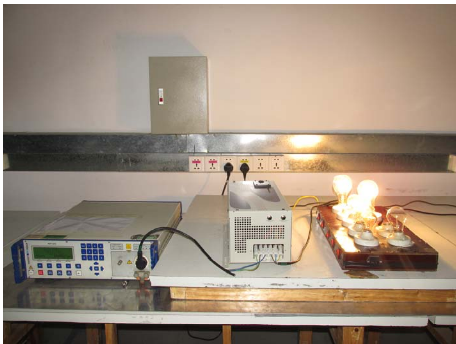
16.6. Photos of Electrical Fast Transient /Burst Test
